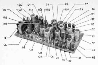
Mounted vertically the components resemble the skyline of a large city. This technique allows more components to be packed into each square inch of perforated board. Wafer-thin C1 is mounted against underside of board.
