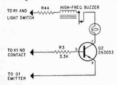
Fig. 3. When using this circuit wire a 10-ohm resistor across buzzer to pass additional current to light lamp 11 properly. Resistor R4A should be 27 ohms, 1/2 watt for a #47 lamp.
