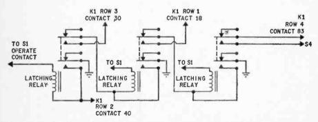
This alternate latching-relay circuit can be carried out still further by adding even more relays. Complex contact combinations can be made with just a little time for experimenting.
