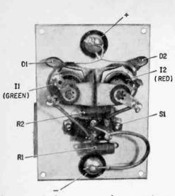
Large terminal screws are for convenience since current is limited by pilot lamps.
