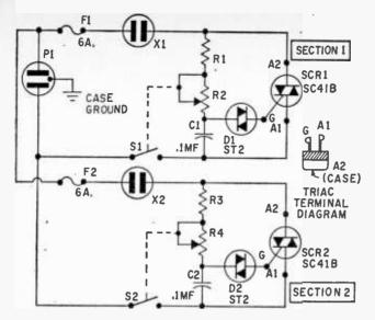
Schematic diagram of the Photo-Trol shows the double circuit—section 1 and section 2—for control of two sets of lights. Each section is rated at 6 amperes or 700 watts. Details for increasing the power capacity are given in text. Use of plug P1 on the chassis box allows the box to be mounted on your tripod with no permanently attached external power cables to get in your way.
