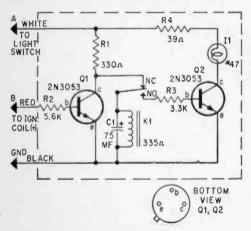
Fig. 1. In the circuit above, capacitor C1 can be increased in value to slowdown clicking of relay K1 and flashing of warning lamp 11.
