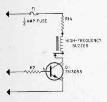
Fig. 2. Resistance R1A (1000 ohms) limits current through the high-frequency buzzer and drops the voltage so that rated value is measured across high-frequency buzzer terminals.
