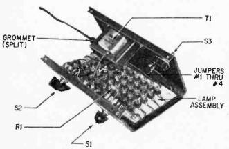
Completely wired unit is ready to be "buttoned up" after final check has been made. Grommet is split to go onto ready-wired linecord of T1. Put a knot in linecord to give some strain relief to the connections on T1. Cord protecting grommet fits in slot in edge of side of cabinet's bottom plate.
