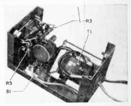
to Normal. Adjust the multimeter Ohms-Adjust knob for a reading of zero ohms. Set the Expander to X100K. With a screwdriver, set R4 so that the multimeter again reads zero ohms (this adjusts the voltage to 67.5 volts and shouldn't have to be touched again unless the line voltage changes). Plug the meter leads into the Expander, connect a resistor, press the Read button, and read.
