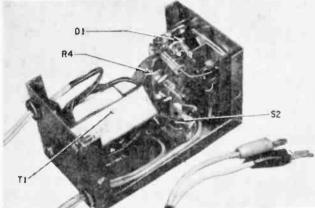
For some multimeters (VOM's) you'll need pin tips on the leads instead of the banana plugs shown here. Since some connections are quite close together it is best to use plastic sleeving (spaghetti) on the longer pigtail leads.
