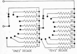
Fig. 2. Nine resistors and a single-gang selector switch are needed for a decade.
