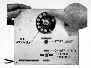
Make all your tests before installing Dial-Lock in partition. You can use lamps in place of the alarm bell and electric door latch for testing. Schematic diagram of the power supply (below) shows how various voltages are taken from unit with a common ground terminal.
