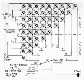
Wiring of Calculator is quite simple. The ten lamps of Circuit #2 are physically fitted into the vacant triangle in the lower-right corner of Circuit #1.53 can be replaced with a pushbutton or eliminated since the NC positions of \$1 and \$2 have the same effect. For a much brighter display use 6-volt pilot lamps—replace T1 with 6.3-volt filament transformer and eliminate R1. S3 should be a momentary contact pushbutton to give long life to pilot lamps.
