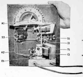
dialed 778-99 for a total of 40 contacts after the START contact in ROW 1; the wiper arm is on the latching-relay contact.
