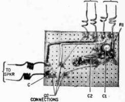
mine the output frequency(s) to some degree, C2 has the greatest effect. The specified value of .02 mf. produces a high pitched tone just about equal to that of the new police type electronic sirens. To lower the tone increase C2's value; to raise the pitch decrease C2.—any value from .01 to .1 mf. will work.
