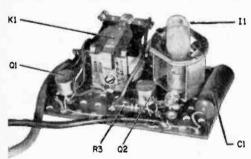
Fig. 4. Basic parts layout may seem a bit crowded—parts placement is not critical. Pilot-lamp jewel bezel threads into ring of pilot-lamp assembly that surrounds lamp 11.
