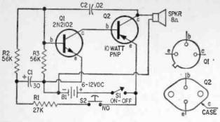
Capacitor C2 provides the necessary feedback to bring the audio amplifier circuit into oscillation. Try different values for C2 (see text) to alter the Screamer's ouput pitch.
