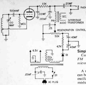
plugged in and connected to a ground. Reverse the AC plug prongs so the lamp does not light. Keep the regeneration control so that the circuit won't oscillate and cause interference. The set will be most sensitive just below the point where oscillation begins.
