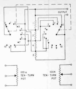
Fig. 1. Circuit of resistance substitutor. Fig. 3. (top, right) Four resistors and a 2-gang switch form one resistance decade. Fig. 4. (above) Potentiometer-type circuit.
