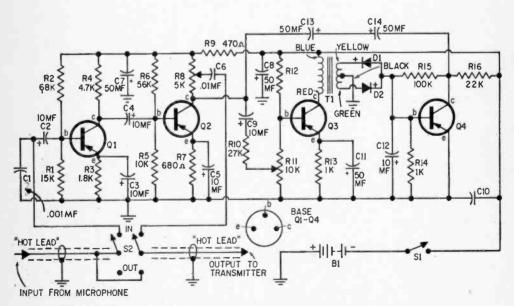
Switch S2 can be eliminated if you want the Compressor to be in the circuit at all times.
