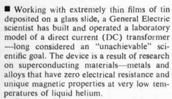
General Electric physicist Dr. Ivar Giaever disclosed that his DC transformer, which can convert a direct current input into a larger or smaller direct current output, has been operated at very low voltages and currents with an efficiency of about ten per cent. Although no immediate commercial applications are foreseen for the DC trans-
