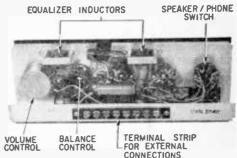
Shot of Control Center with cover removed shows wiring, controls, and terminal strip for connecting both amplifier and speakers.
